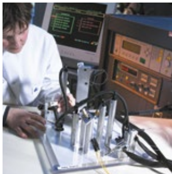
▲ AUTOMATIC CONTINUITY & INSULATION RESISTANCE TEST
