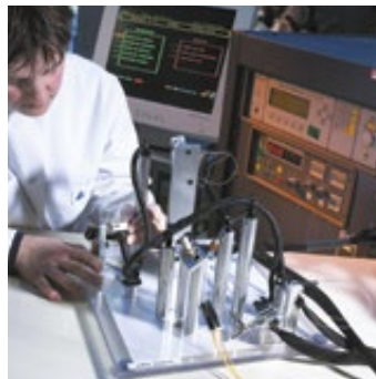
▲ AUTOMATIC CONTINUITY & INSULATION RESISTANCE TEST
